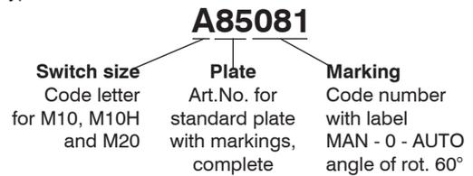
However, if a **switch** with non-standard lettering is required, only three-digit code number for the marking need be added to the order type (see next page).
