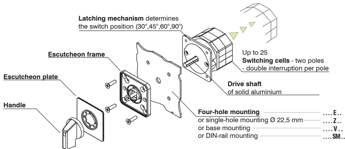
1) Control Switches with double contacts for highest contact reliability.
