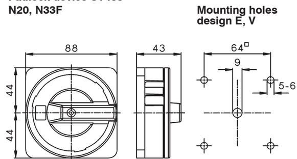
**Front plate/switch shaft sealing FPWD**
