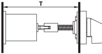
Door couplings are available for switches to be installed in switchgear cabinets or distribution boards with hinged doors. These permit the doors to be opened without removal of the operating knobs.
